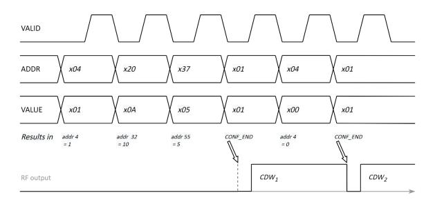
Figure 2: Example of CDW parameters at the FCP interface and their interpretation. Figure not to scale.
